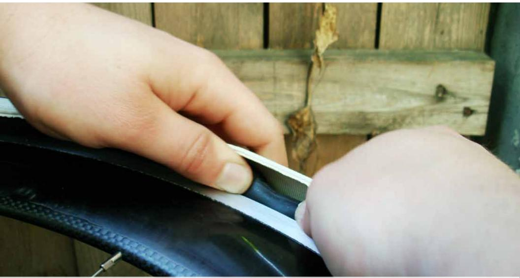
As you get the last part of the tube in the wheel, which should be at the opposite of the valve you can use your forearms to keep the tire down to prevent the tube from popping back out.
