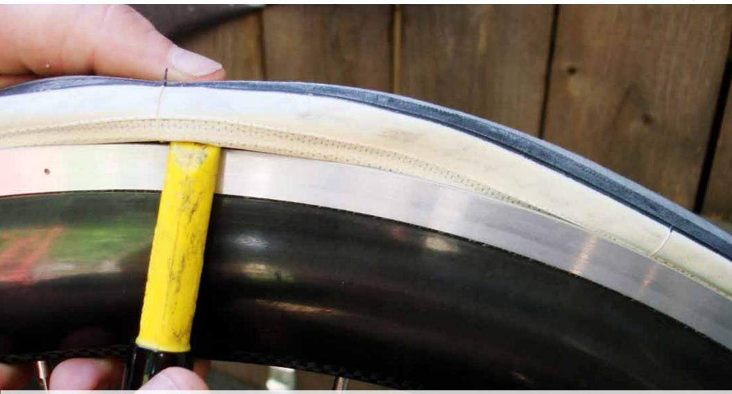
Push lever down over the rim to force the tire's bead to jump over the sidewall.
