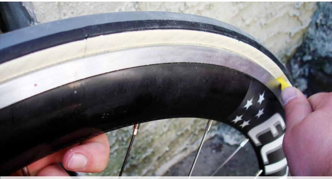
After the lever is positioned properly, simply slide(may be difficult to start, but with a little momentum it is easier) the lever down the rim to let the bead jump accordingly onto the wheel. Be sure not to lift the tire lever over 90 degrees to the rim as you can catch the tube and rip a hole in it as well. After the tire is on, run around the rim pulling the tire back a little, if there is tube exposed, massage the tire until the tube disappears into the tire.
