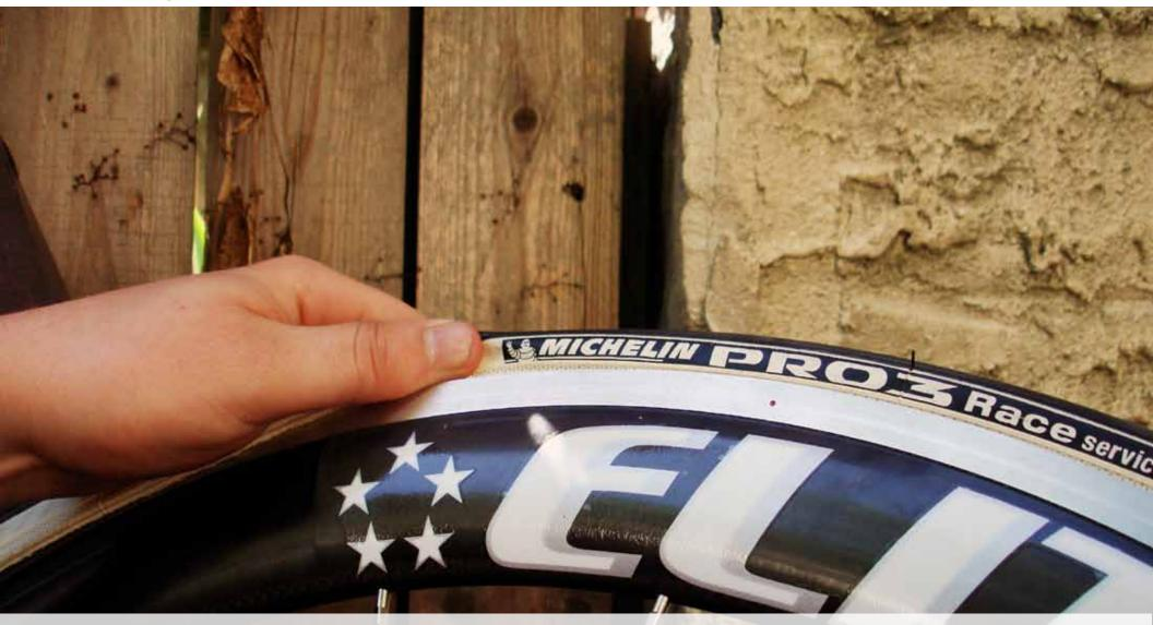
Moving on to put the tire back on completely to the wheel, again, start at the valve. You may have to push the valve up a little to allow the tire's bead to jump underneath the sidewall properly. This process should start there and move both ways down the wheel to end on the opposite side of the valve.
