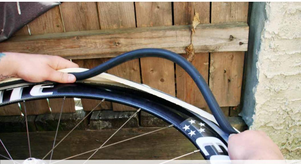
As you push the tube in, be sure to run both ways around the rim to keep the tube from pulling from one side or the other and pulling the valve away from coming straight out of the rim.
