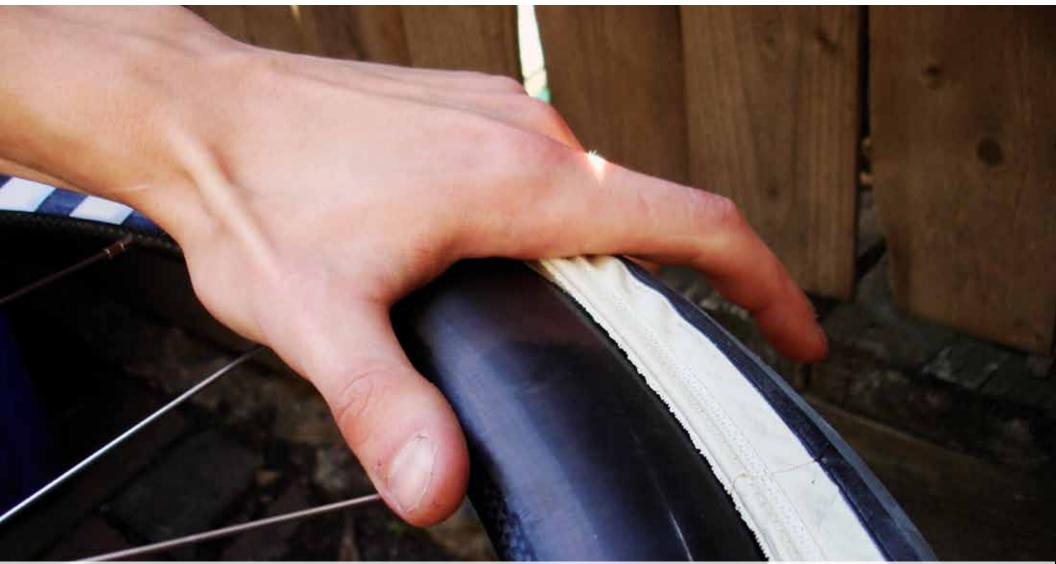
As you get closer to the end of getting the tire on, it will get increasingly harder to push the bead over the sidewall. This is where a little elbow grease comes in handy, a useful technic is to use inside of your knuckles on your hand and somewhat roll the bead of the tire back over the lip of the sidewall, going back and forth between both ends of where the bead is still exposed and working towards the center.
