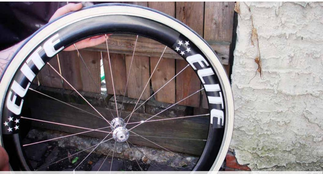
Here is the tire with one of the beads on the outside of the rim, so the tube is ready to be extracted.
