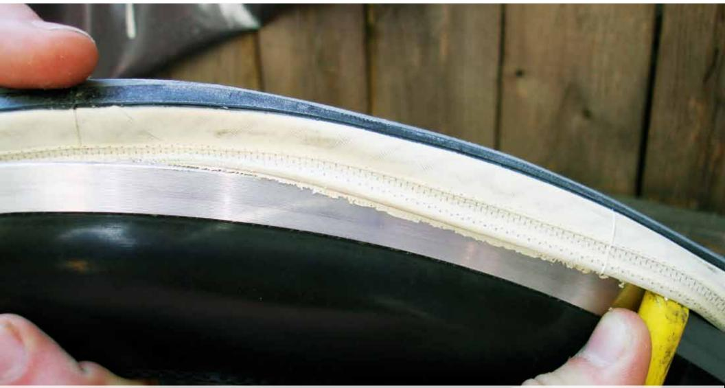
Once the tire is popping over the rim, push(or pull, whichever is easier) the lever along the rim making the tire bead jump more and more over the sidewall on the outside of the wheel.
