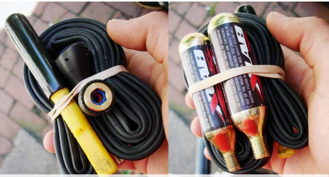
Here is an example of a decent repair kit setup that we suggest. It contains a tube, tire lever, inflator, and two  $CO_2$  canisters. There are several different ways to carry a tube with a small pump or different kinds of inflators, whatever works best for you may not be this, that's fine.
