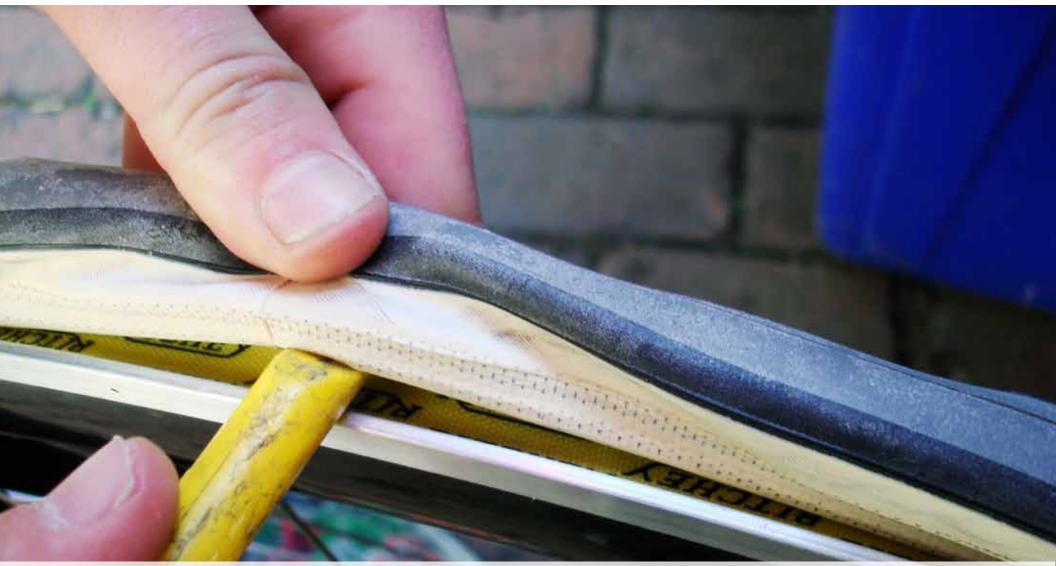
Use the groove on the tire lever to grab the bead of the tire itself in order to pull the tire over the sidewall of the rim.
