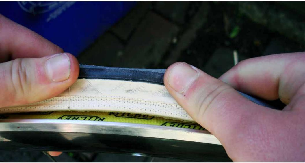
Begin then by peeling back tire bead from rim(in some situations you may need to push bead off of entire rim to loosen tire from wheel in order to make it easier to get off) to make room for the tire lever to fit inside.
