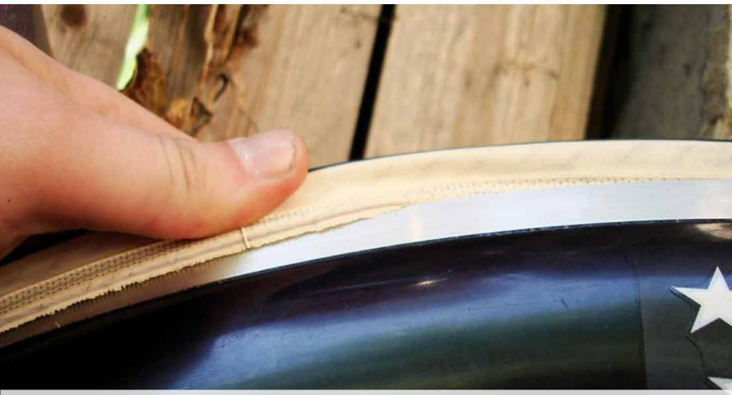
You can use whatever part of you hand that you need to push the bead properly over the sidewall and get the bead under the lip of the sidewall as shown here using his thumb.
