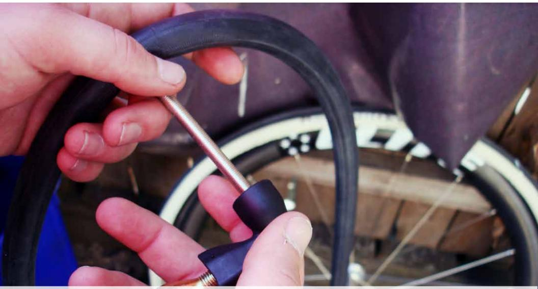
After unpacking your new tube, grab your  $CO_2$  canister with inflator attached. The way these work is that the canister gets twisted entirely into the inflator(which both punctures and seals canister)
