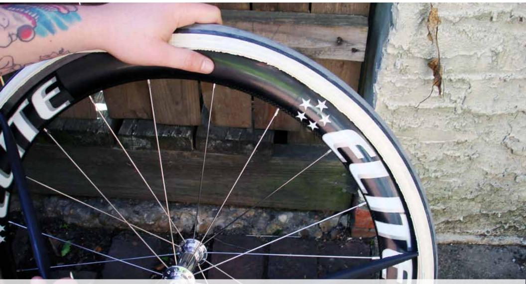
Start opposite the valve and simply pull the tube away from the tire and rim.
