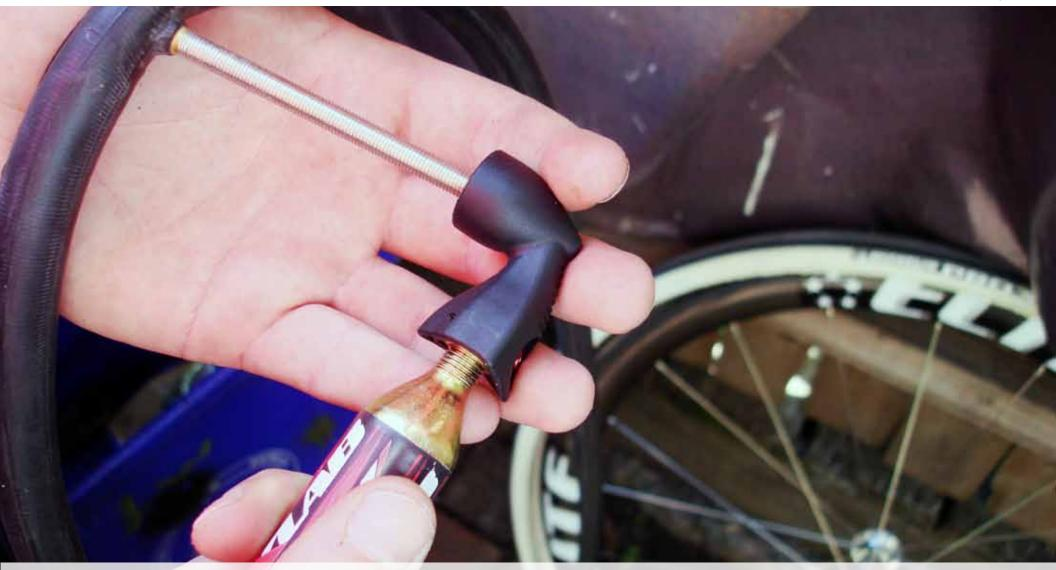
And then untwist it slightly for a moment to allow enough air into the tube to give it a little bit of shape. If you have a pump, one or two pumps should suffice how much air should be in the tube to begin. This is done so that the tube will go into the tire easier and not get pinched during installation.
