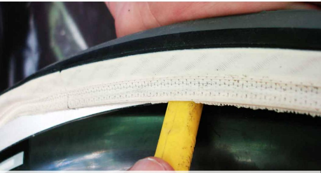
Slide the tire lever under the tire with the cutout facing the rim this time and the smooth part towards the tire. Be sure to not get the tube in between the lever and the sidewall of the rim as you will pinch the tube and rip a hole in the tube itself and have to start all over.
