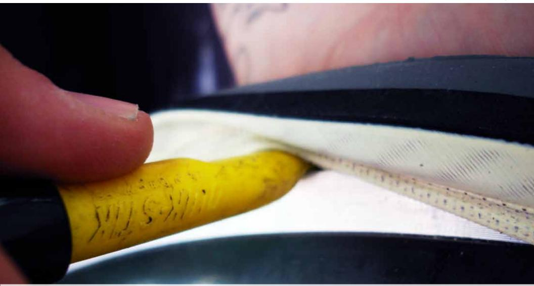
Lift the lever up to have the one side of the bead pop over the sidewall.
